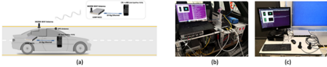
Figure 90: SDR-based V2X communication device on TUC vehicle platform: (a) installation setup (b) UE (c) CN+eNB
