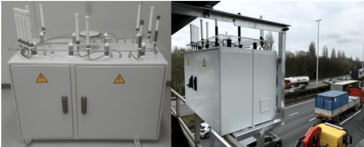
Figure 83: RSU on E313 highway
