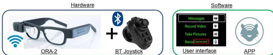
**Figure 11: The components for the Smart Glasses to be used in the Enhanced Experience**
