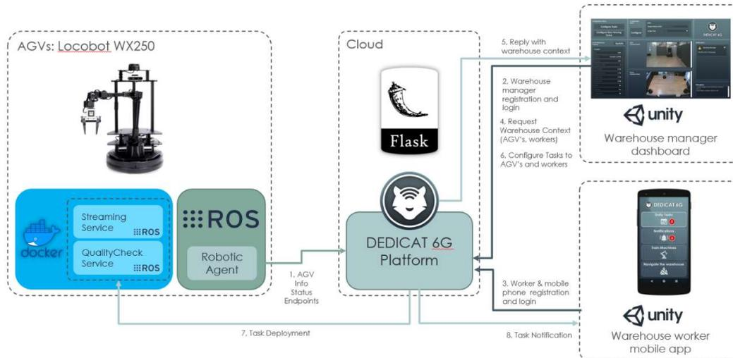
**Figure 10: View of the smart warehousing implementation**
