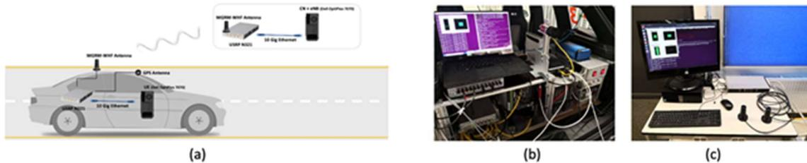
**Figure 36: SDR-based V2X communication device on TUC vehicle platform: (a) installation setup (b) UE (c) CN+eNB**
