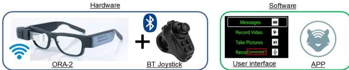
**Figure 19: The components for the Smart Glasses to be used in the Public Safety use case**
