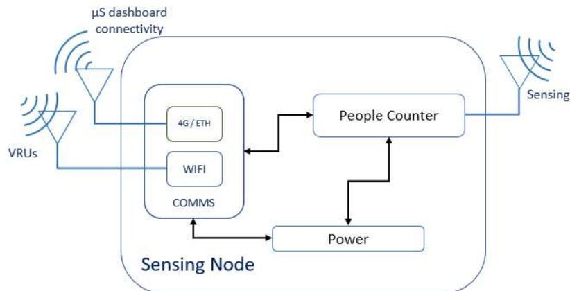
**Figure 38: Sensing node prototype**
