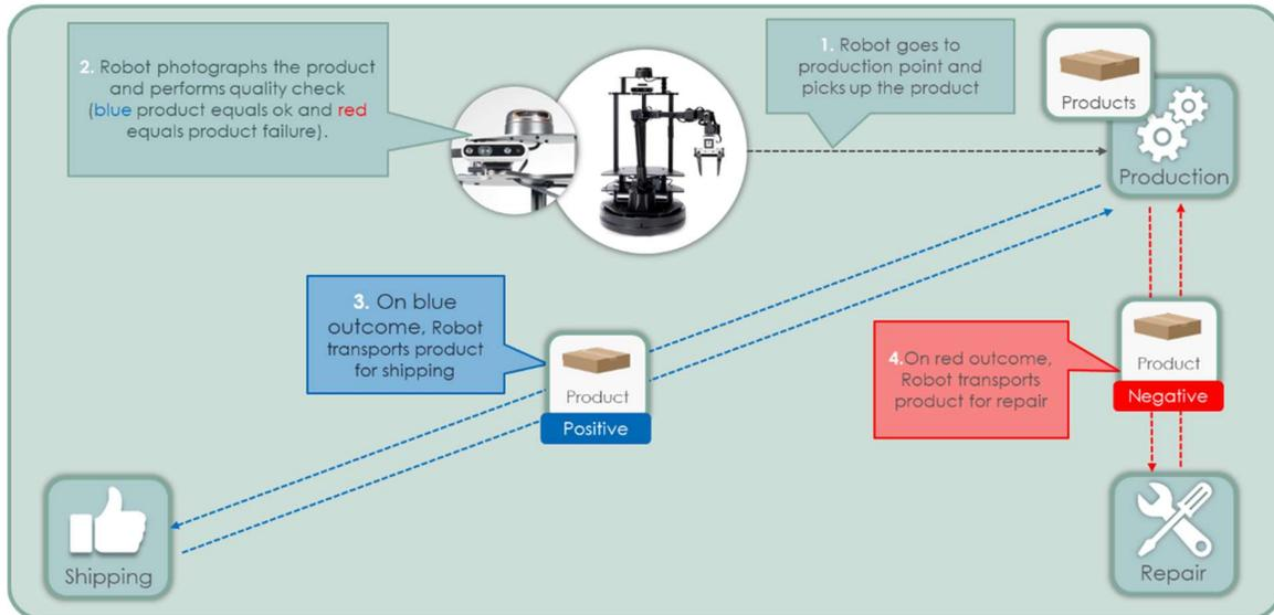
**Figure 6: Indicative quality check scenario in the scope of Smart Warehousing**
