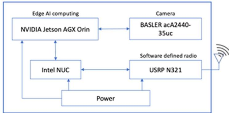
**Figure 33: RSU prototype hardware configuration**
