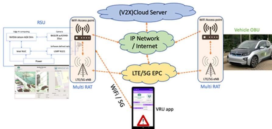
**Figure 37: End-to-End Network for UC4**
