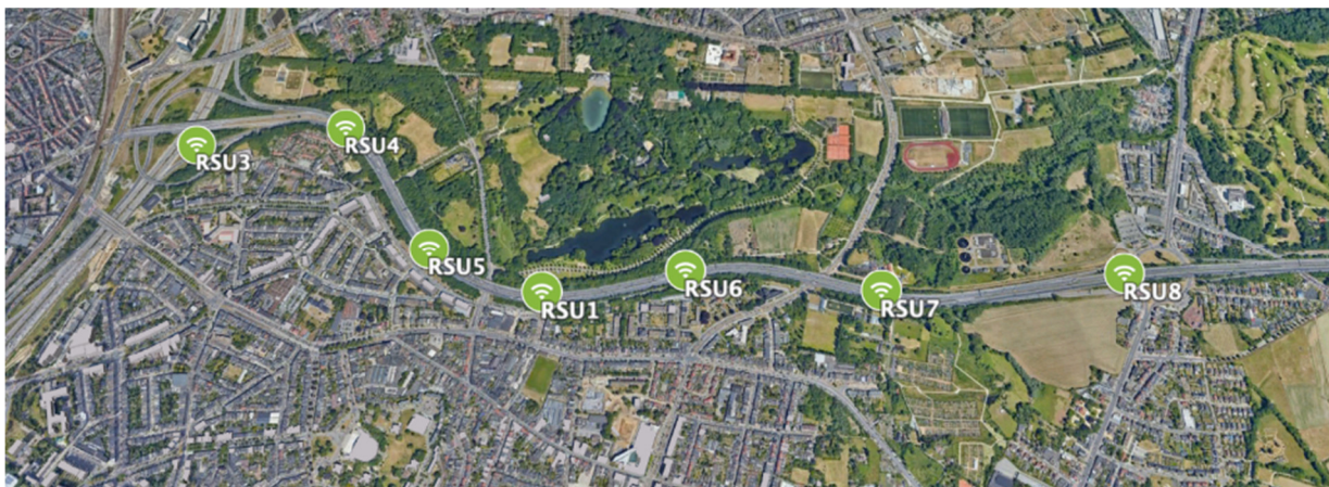
Figure 10: RSU locations of the Smart Highway testbed along the E313 highway
